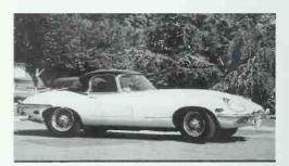
This 1969 Series II 4.2 perfectly illustrates the exterior alterations for the U.S. market: grille bar as part of bumper; amber signal lenses under the front bumper; amber side flashers; headlights moved forward with wide chrome band covering the gap; hex-nut knockoffs; amber side flashers below rear bumper; exhaust pipe angled out around rear license plate mount. This car has the accessory removable hardtop and an aftermarket luggage rack. *Jaguar Journal*
