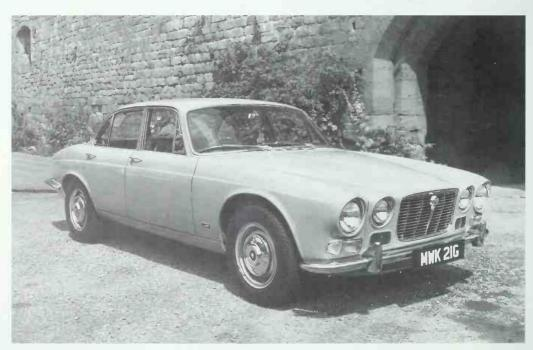
UK factory press kit shot of the original Series I XJ6. Round badge at top of grille is Jaguar head. Note low bumpers, signal/parking lights with white and orange lenses, plastic leaper on front fender. This
