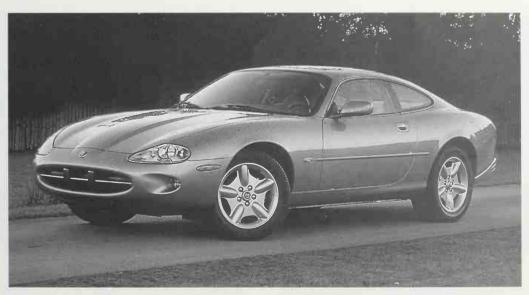
XK8 Coupe. All details and equipment are the same as the convertible. Rear door is a lift-up hatch and the rear seat folds to give a long luggage platform. *Jaguar Cars*
