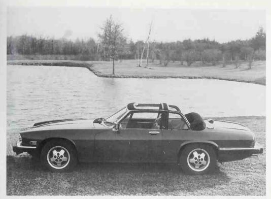
Side view of 1986 Cabriolet with different angle on the top rails. These cars had the same frames around the side windows as the coupe. No frameless door glass on the XJS until the full convertible of 1988. This view also shows the little leaper on the B
