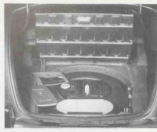
Useful shot for show competitors showing 3.8 "S" handbooks with plastic envelope and the tool kit recessed into the spare wheel. This method of stowing the tool kit was used on the whole "Mk 1" and Mk 2 series as well as on the E-type. As usual, the spare wheel well is a prime candidate for rust. *Jaguar Cars*
