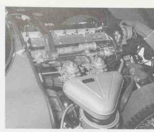
Series II E-type engine compartment showing two Stromberg carburetors on exhaust-heated inlet manifold. Polished thick tube coming over the rear of the engine carries exhaust heat. Square tubes for engine/suspension sub-frame can be seen to right and left of the triangular air chamber which sits above the round air filter housing. *Jaguar Cars*
