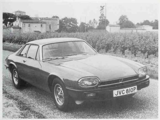
The original 1976 XJS in UK form with single unit headlights and missing the outside rear view mirrors. These lights were often installed by owners in North America, even though they were not federally approved. Note V-12 badge in grille center,
