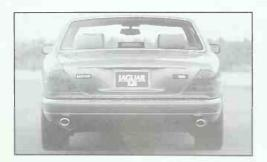
Jaguar XJR, supercharged sedan. Rear view shows new tail lights common to all 1995 sedans, new trunk lid with recessed license plate mount and body color lock/lamp housing. Other 1995 Jaguars have chromed housing. Small round Jaguar head is electric push-button to release the trunk latch. Name plates for other models are similar. Jaguar Cars
