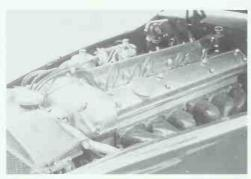
Under the hood, this later XK 120 has the corrected cam covers with bolts holding the leaky forward portion down. Vitreous enameled exhaust manifolds can be seen. This attractive finish unfortunately flakes off due to expansion and contraction. *Karen Miller*
