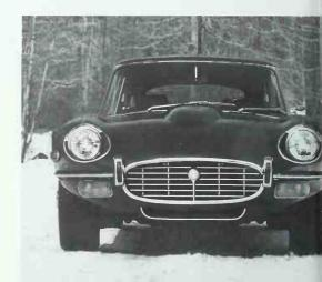
The aggressive front of the 1971 V-12 2+2 E-type. The grille and Jaguar head badge are clearly visible as are the usual amber sidelights and below-bumper signal/parking lights. The small rubber-faced chrome bumper guards lasted only one year. Jaguar Cars
