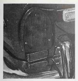
Detail of Series I XJ12 tail-light showing edge of backup light, extra reflector to meet U.S. reflector area requirements, typical Series I and II cathedral tail light lens. *Jaguar Cars*
