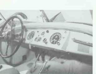
The XK 140 dashboard is very like the XK 120. However, the flat steering wheel center/horn button, immediately identifies this as a 140. *Karen Miller*
