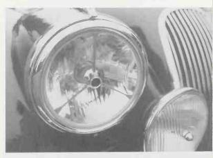
Detail of XK 120 front end shows Lucas tri-bar headlight unit, accessory fog light and assembled grille. Each vertical bar was individually attached to the grille shell. Karen Miller
