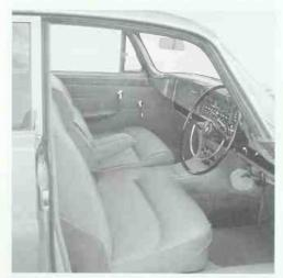
Driver's side view shows plushy seats—not buckets but individually adjustable, cane-type handbrake, radio speaker. *Jaguar Cars*
