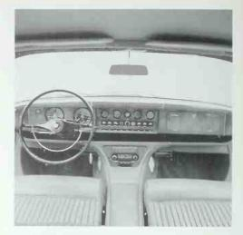
Interior view with seatbacks reclined gives unobstructed view of dashboard showing console with pull-out tray and radio installation. Fussy, narrow seat pleating appeared on Mk X and 420. Jaguar Cars
