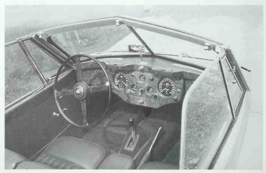
XK 140 drop-head interior. All-wood dash has dual ashtrays on upper edge, storage drawer at lower
