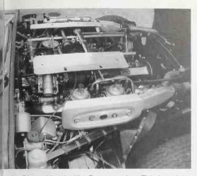
Right side of 1974 E-type engine. This is a righthand drive car so the master cylinders are on this side. The battery is installed on this side and you also get a view of the fiber-board water deflector installed just forward of it. You can also see the air injection rails, straight silver pipes running fore and aft with smaller pipes going straight down next to each spark plug. *Mike Cook*
