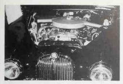
Under the hood of a 1966 3.8 Mk 2 belonging to John and Mary Lou Splitorff showing the very different later air cleaner with dual intake pipes going to the carburetors. 3.8 heads are painted dark metallic blue. *Mike Cook*
