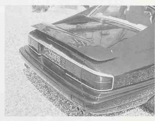
Rear view of the XJR-S showing wrap-around rear bumper and valance panel, trunk-mounted spoiler. John Crawford
