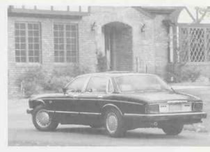
1992 Vanden Plas Majestic with new wheels for that year. This shows the chrome trim added to the rear of the trunk lid, across the bottom of the rear panel and around the tail lights. On the side, the upper chrome strip is standard on VDP. The lower, wide chrome strip was unique to the Majestic. *Jaguar Cars*
