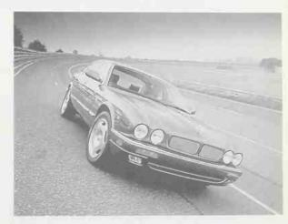
Front view of XJR shows body color grille surround and steel mesh grille panels. Mirrors are also body color. Wheels are 5-spoke alloy with 17-inch rims. Jaguar Cars
