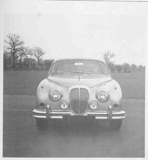
Front view of Daimler V-8. The appearance is identical to the Mk 2 except for the wider, fluted top of the grille.
