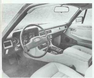
Adding burl elm trim to the H.E, interior made it considerably brighter. All switches and instruments are the same but the silver trim was deleted from the instrument panel. The seat upholstery is no longer perforated. Rocker switch at the end of the shifter housing is for cruise control. This view also shows the rear ashtray on the back of the arm rest. Plastic housing visible on the door post at left houses the fuel shutoff switch. *Jaguar Cars*
