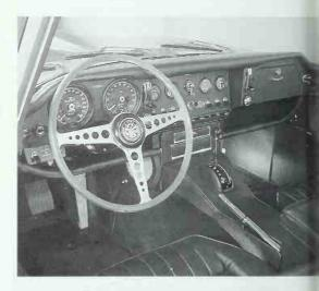
1966 Series I E-type 2+2 dashboard. This is a late model with the add-on Hazard Warning switch panel at the left of the dash. Two levers to right of the tachometer control footwell air flow. Lever to right of center panel is the choke. Note automatic selector. The brake pedal is larger than the one fitted to stick shift cars. *Jaguar Cars*
