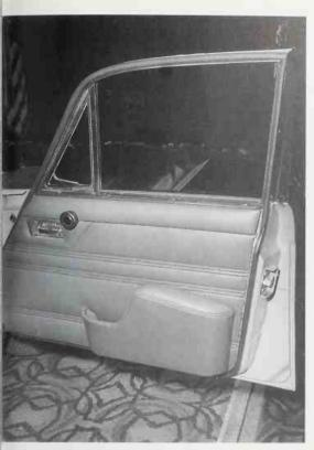
Original Series I XJ6 door panel. Knob opens quarter window. Lever in front of door handle is the lock. Arm rest has pocket. Note no window control—switches are on console. *Jaguar Cars*
