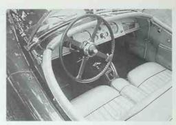
XK 120 interior details showing central instrument panel which allowed building right or left-hand drive cars without too many production changes. Padded panel on the driveshaft tunnel often accommodated a third person in those days before seat belts. *Karen Miller*
