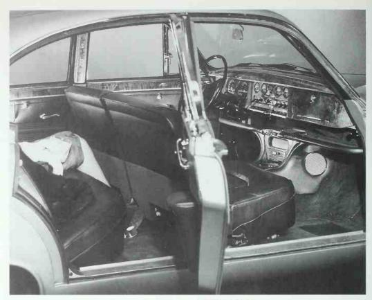
3.8 "S" interior. Wood trim extends up both A and B pillars and across top of dash. No radio in this stick shift car. This was a factory advertising photo but the ignition keys are hung on a piece of string! Note notch in the center of the parcel shelf which holds direction controls for heat/defrost. Rear legroom is demonstrated by person sitting behind the driver's seat. Jaguar Cars
