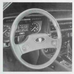
1989 dashboard showing different steering wheel with sculptured finger grips and separate horn buttons. This wheel was used through 1992. Electric seat heater and lumbar support controls are on the side of the console. The seat and seat back still adjusted manually. *Jaguar Cars*
