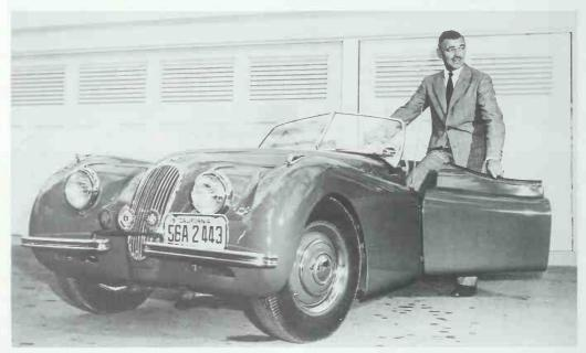
Specifications on Clark Gable aren't available but this photo shows some good details on his new XK 120. This early car has the separate chrome-plated, parking lights on top of the fenders and lacks the footwell air intakes. The disc wheels were standard
