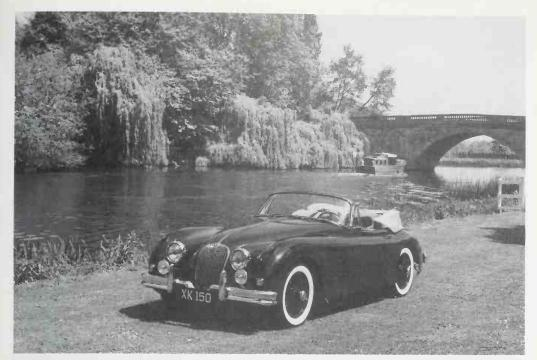
XK 150 drop-head with body-color wire wheels, Much wider hood can be seen, together with full-width bumper, wider grille, *Jaquar Cars*
