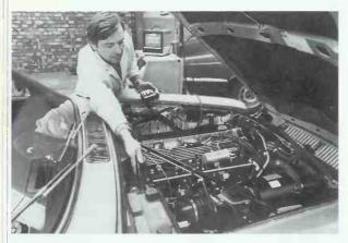
U.S. specification XJ6 Series III engine on emissions test at the factory. This is the fuel-injected, 4.2 engine. *Jaguar Cars*
