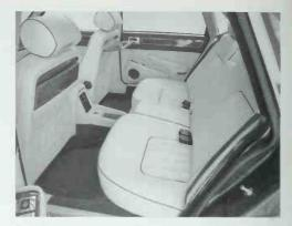
Majestic rear seat showing typical Vanden Plas picnic tables and central console with heat/A/C outlet. VDP rear seats were constructed as two "chairs" although a seat belt was provided for a center passenger. The fold-down armrest is visible. On the VDP there is also a "secret" storage compartment in the center cushion. Small map lights are in the back of the headrests. *Jaquar Cars*
