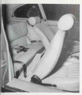
Back seat of Series II 2+2 coupe. Seat looks good but footroom is virtually nil. Detail of front seatback adjuster is visible, as is the ashtray on console with black crackle lid and small leaping cat emblem. Jaguar Cars
