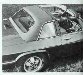
Seldom seen picture of XJ-SC "hardtop" in place. The rear section was molded fiberglass, covered in fabric to match the removable front panels. The car could be ordered with just the hardtop or with the folding rear soft top section as well. *Jaguar Cars*
