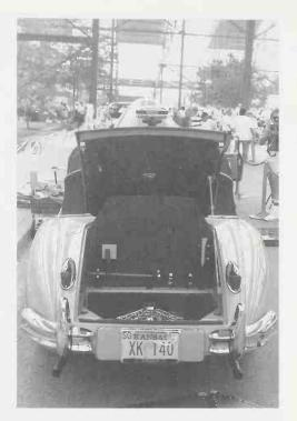
Rear view of XK 140 showing hardboard spare tire cover with grease gun and jack clipped to underside, double latches on trunk lid, light under lid and painted rod to prop lid open. Heavier 140 bumpers can be seen. This is the 6-time national champion drop-head owned by Jack Stamp. *Karen Miller*
