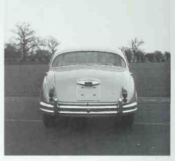
Rear view of Daimler V-8 with chrome script on right lower corner of trunk lid. The license plate/backup light housing also has the Daimler fluting. A small, round "D" badge is in the center of the bumper where Jaguar Mk 2s have a "disc brake" badge. Jaguar Daimler Heritage Trust
