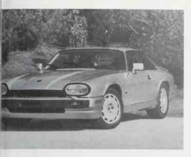
The 1993 XJR-S. Seen from the front are the molded bumper/spoiler, single unit headlights, headlight washers and 16-inch special wheels. *John Crawford*
