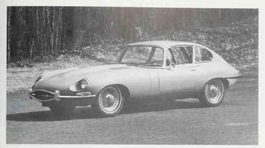
A 1968 2+2 Series I without headlight covers. The headlights are still in the original position—Series II lights were moved forward in the nacelles. The federally required door mirror and
