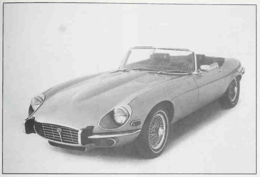
1973 E-type Series III showing bumper guards unique to that year. They are rubber over steel
