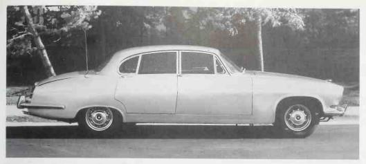
Mk X fitted with later XJ chrome "Turbo" wheels. Roof and side window styling carries over from the Mk IX but everything is larger, especially the front
