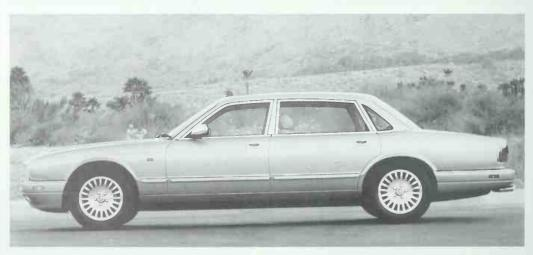
The extended wheelbase 1996 Vanden Plas. The extra width of the rear door is visible as well as the altered rear pillar behind the quarter window. *Jaguar Cars*
