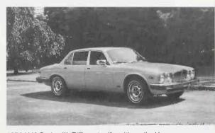
1979 XJ6 Series III. Different grille with vertical bars, flat roofline, larger side glass and windshield, two mirrors and flush door handles are all visible. The 1979 and 1980 XJs had full, chrome-plated wheel covers with fake bolt-heads. From 1981 on, they used original XJS alloy wheels. *Jaguar Cars*
