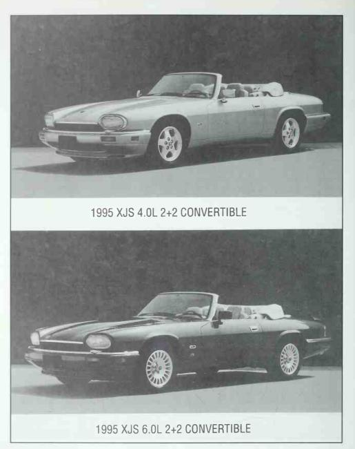
Paired shot of 1995 XJS 4.0 and 6.0 liter convertibles. They are identified as 2+2 because, in 1995, a rear seat was provided in the convertible for the first time. Wheels are different, the 12 has the headlight sur-
