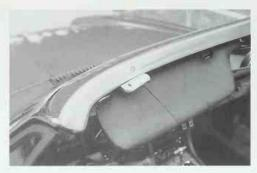
Attachment plate for H & E convertible top which rests on top of the windshield frame rather than attaching from the rear like the factory top. Portion of roof between the windshield surround and the polished chrome header trim is painted body color. *Mike Cook*
