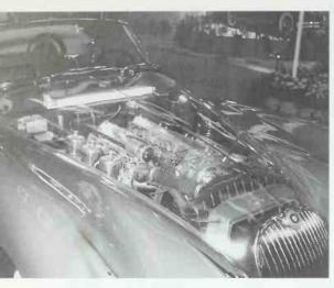
The XK 150 "S" came in 3.4 and 3.8 liter high-performance versions with triple SU equipped engines. This New York show car with clear plastic bonnet displays the tri-carb installation, wider grille, enamel badge reading "Jaguar XK 150" with the Jaguar head in the center. Needless to say, production cars did not have this gleaming finish. *Jaguar Cars*
