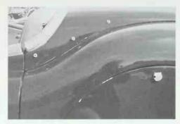
Detail of XK 140 roadster showing cockpit edge trim, top snaps, narrow black fender beading and Dzus fastener for fender skirt. *Jaquar Cars*
