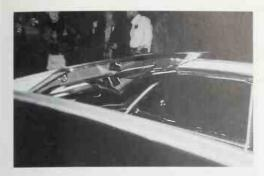
The 3.8 Mk 2 of John and Mary Lou Splitorff has a Webasto fabric sun roof which opens over both front and back seat. A large plastic deflector pops up when the roof is open to reduce buffeting. Rarely seen, the Webasto unit was factory approved and could be ordered as original equipment. This shot also shows wood trim on B pillar and above door. *Mike Cook*
