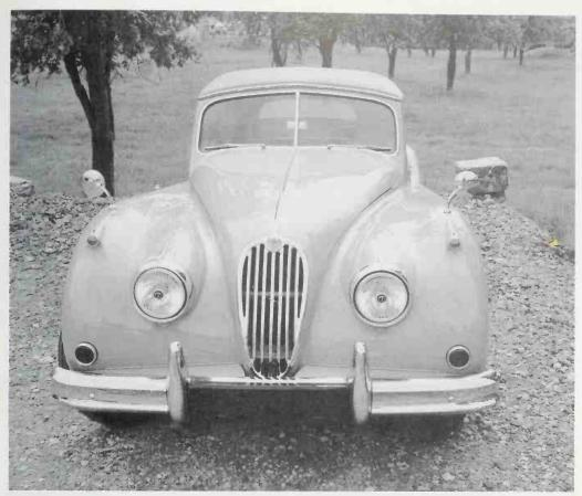
Front view of XK 140 shows one-piece die-cast grille with heavier bars than XK 120, heavy bumpers and thick windshield pillars. The grille
