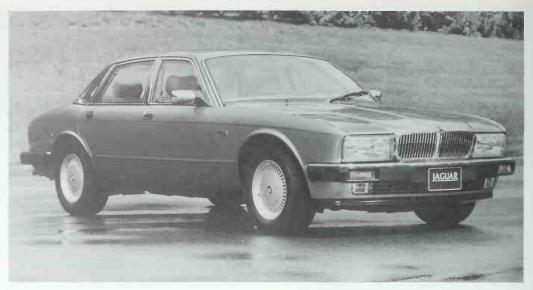
1993 XJ6 showing new style wheels that year. The front panel below the front bumper was new, incorporating fog lights beside the air intake. *Jaguar Cars*
