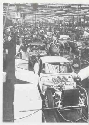
Factory production line shot showing three-carburetor engined cars. This angle clearly shows the sub-frame construction including forward supports for the radiator. The car's narrow track is apparent. *Jaguar Cars*
