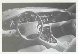
XK8 dashboard. Main gauges are in front of the driver. Auxiliary gauges are in the center panel. Righthand walnut panel covers passenger's air bag. Glovebox is below the panel. J-Gate controls ZF five-speed automatic. Cruise control buttons are on steering wheel. *Jaguar Cars*
