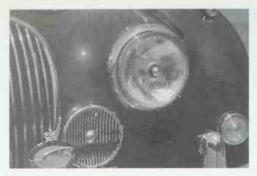
Detail of Mk 2 showing tiny parking light on top of fender, round signal light, horn grille. Jaguar Cars
