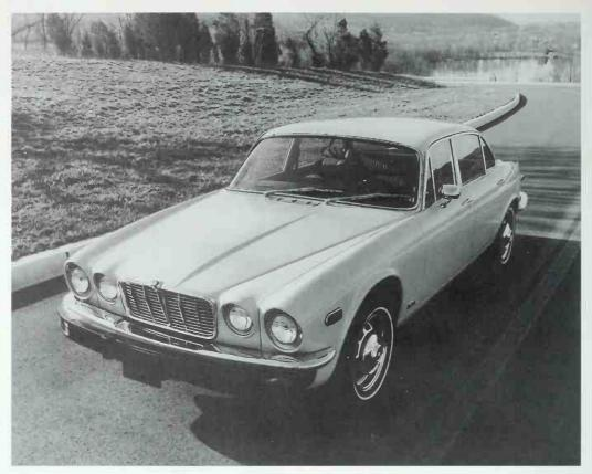
1975 Series II front showing altered grille with painted vertical bars, heavy rubber bumper with signal lights in the ends, chrome trim on bumper. Still no standard
