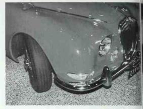
Front corner of 3.8 "S" belonging to Pat Shasby. The style is similar to the Mk 2 but note slim bumpers, wrap-around signal lights and eyebrows over the head and fog lamps. The lights are set into the panel without chrome rims. There are no parking lights on top of the 3.8 "S" front fenders. *Mike Cook*
