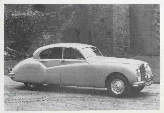
The Mk VII sedan. It shares the side fender line with the XK 120 but carries the Mk V roof and side window styling and has a two-piece windshield. Despite
