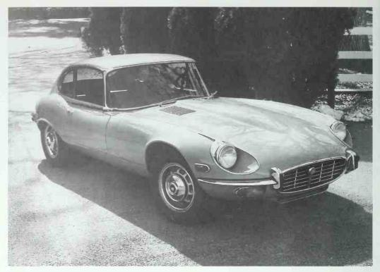
A rather pleasing view of the Series III 2+2 showing the standard, painted Turbo wheels and small, 1971 bumper guards. This picture also illustrates the high
