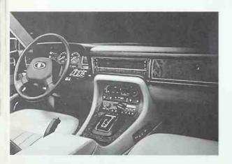
In this photo of the 1988 XJ sedan, the dash lights are on and a corner of the VCM warning can be seen at the right of the instrument panel.
