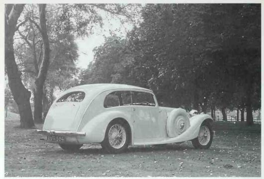
The Airline's most distinctive angle, showing the unusual shapes, of the rear side windows and back window. The car had a drop-down trunk lid, center-mounted tail-light unit and chromed drip moldings extending
