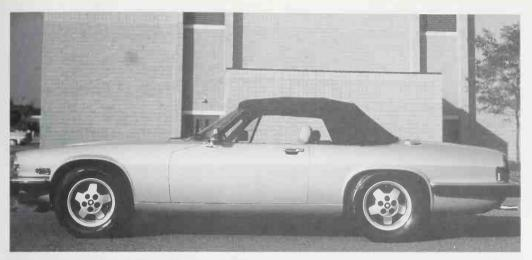
1987 Hess & Eisenhardt convertible. This side view shows how the top drops down on top of the windshield. Side section of top wraps around further than
