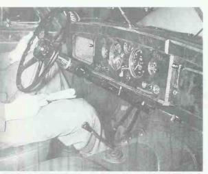
Dashboard of original 1955-59 2.4 or 3.4 sedan. This illustrates the centrally located instrument cluster which allowed British car manufacturers to build right or left-hand drive cars with minimal interior change. For a right-hand drive car, only the locking glovebox and open "cubby" box would change positions. Controls and instruments stayed in the same position. Ignition switch and starter button are at lower right of panel. Levers on either side are for heat/defrost direction. Jaguar Cars
