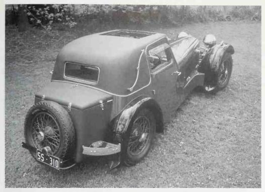
A rear view of the original S.S.1 with "helmet" front fenders and no running boards. The sun roof is open
