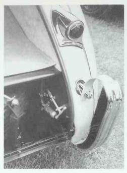
This is a detail of an alloy-bodied XK showing the trunk mat, separate spare wheel compartment and wheel clamp arrangement. Clipped at the right are the grease gun and the "T-key", used to lock and unlock the fender skirts. On steel-bodied cars, the lower portion of the fenders, the compartment floor and little nooks and crannies in the rear bodywork are all subject to rust. Mike Cook
