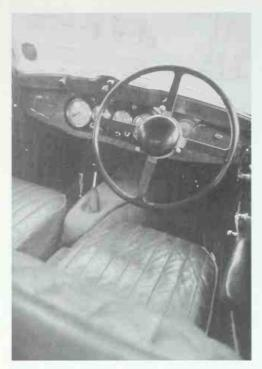
Interior of the 1937 S.S. Jaguar 2.5 liter saloon. Instruments are now housed in a black panel set into the wooden dash. Center crank opens the windshield. Large knobs on either side are individual wiper controls. On the steering wheel hub, the turn signal control is at the top. This is basically an original car with leather in excellent condition. Paul Skilleter
