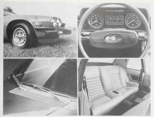
Four detail shots of the original XJS: front end showing painted alloy wheels, flexible front spoiler, dual U.S. headlights; Instrument pack with unusu-
