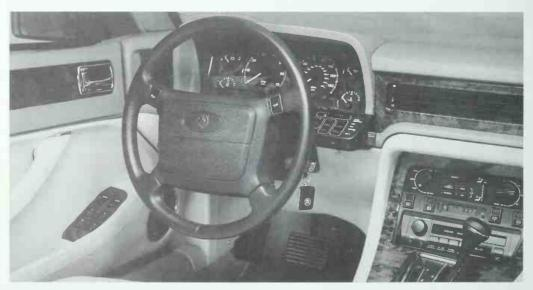
1993 interior showing new steering wheel with air bag and horn buttons on upper spokes. The instrument panel is the 1990 revision with all round dials
