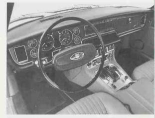
Series II dashboard, also common to Series III. Minor instruments have been moved to either side of the speedo and tach, replaced by the very desirable center A/C vent. Rocker switches are replaced by rectangular push-buttons above the radio, flanking the clock. Heat and A/C controls are still on either side of the radio. Rocker switch on console is for the sun roof. Jaquar Cars
