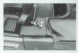
H & E shoulder belts were guided through this finishing panel. Note how flat the folded top is. The cover was vinyl fabric rather than cloth finish on the factory convertible. Carpeted luggage platform has storage under lift-up lid. Radio speakers were in the rear panel. *Mike Cook*
