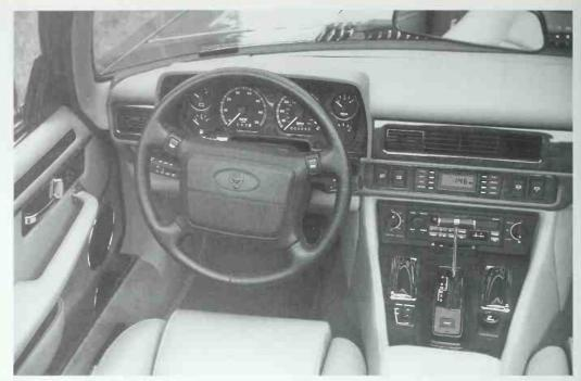
1993 XJS dashboard. Identical to the 1992, this photo shows the light switch on the left stalk, seat control
