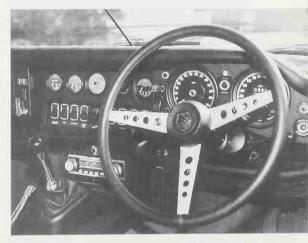
Close-up of the dash of a right-hand drive car. Series III E-types had standard power steering and all were fitted with the smaller, leather-rimmed wheel shown. Spokes are satin silver. Jaguar head is molded black plastic. This non-air car has a UK radio. You can also see the shelf below the dash with its padded edge. *Mike Cook*
