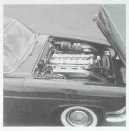
Mk X engine compartment with triple SU carb, 3.8 liter engine. Jaguar Cars
