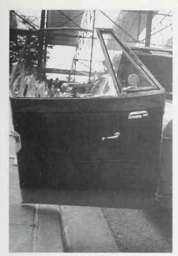
XK 140 drop-head door showing upper wood trim, lever-in-slot door handle and very wide opening door. If the door stop doesn't work, the forward edge of the door will dent the fender. Karen Miller
