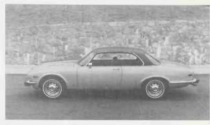
1975 XJ6C showing the roof line to perfection. Note the length of the rear window and the fender space below it and you can see why the lowering mechanism was so hard to perfect. Vinyl roof covering was attractive and good quality but the car takes on new beauty if it is removed and the roof painted. Rear seat room is virtually identical to the four-door. *Jaguar Cars*
