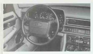
A 1993 XJS dashboard, illustrating the changes introduced in 1992. The wood-veneered instrument panel features six round dials. The trip computer is centrally mounted, flanked by flush switches. The 1993 model was the first to have an airbag on the driver's side. This car is automatic—note cylindrical walnut shifter crossbar. The switch panel forward of the door handle is for power seat adjustment. *Jaguar Cars*
