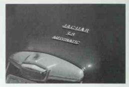
Detail of Mk 2 rear showing model designation, engine displacement and letter indicating the car is automatic. Central back-up light is on license plate light housing. Daimler Mk 2s have "fluted" housing. *Jaquar Cars*
