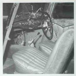
S.S.1 interior showing bucket seats, "sunburst" door trim pattern and extensive use of wood. Speedometer drive cable can be seen coming through the tunnel forward of the handbrake. Note hardware enabling the windshield to be opened, spark and mixture levers in center of steering wheel. The switch in the center of the bottom edge of the dash appears to be an add-on. Jaquar Cars
