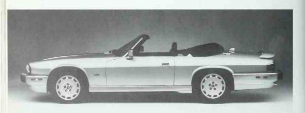
The XJRS came in convertible form as well. This side view shows the body kit, front, rocker panel and rear, plus the trunk-mounted spoiler and special wheels.
