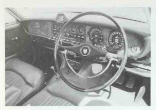
420 sedan interior. The car is stick shift. Note indicator on steering column used to show automatic positions or "Overdrive". These post-1967 cars have padded dash tops rather than wood. The clock is tucked into the edge of the dash pad. *Mike Cook*
