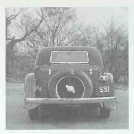
Final S.S.1 from the rear. The trunk is reduced in size and a full width rear bumper, with S.S. emblem, replaces the bumperettes. Eared fuel tank filler cap is at left. The spare wheel cover also has S.S. emblem. The tail light assembly with license plate bracket is typical. Similar units had been used on various Swallow models. *Jaguar Cars*
