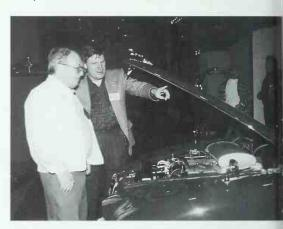
Pat Shasby shows 3.8 "S" to Randy Wright. Eyebrow over headlamp is readily visible. Air cleaner is similar to Mk 2. This car was picked up in England and shipped back—wing (fender) mirror is typical of the period.
