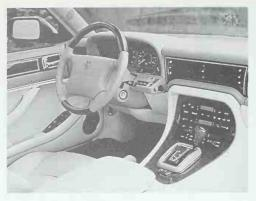
This is the 1995 XJ12 dash panel. Note that the dash top and A pillars are color-keyed as well as the console. The instrument panel is similar to the previous year but the central panel shows new climate control set-up with LED read-out for temperature. Second panel is for the radio. Simplified buttons for the trip computer and cruise control switch are still on the panel to the right of the wheel. *Jaguar Cars*
